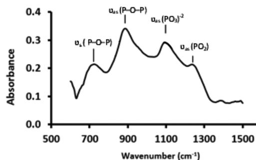
Figure 3. FTIR spectrum and band assignment for PGNs (ν, stretching; s, symmetric; as, asymmetric; δ, deformation).
