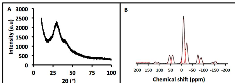
Figure 2. (A) XRD pattern of the PGNs indicate that it is free from any detectable crystalline phase and (B) <sup>31</sup>P MAS NMR spectrum (black line) and the fitting (red line) that correspond to mainly Q<sup>1</sup> and Q<sup>2</sup> phosphate units.
