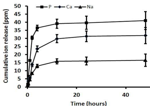
Figure 4. Cumulative release of phosphorus, calcium, and sodium in deionized water as a function of time for the investigated PGNs. Error bars represent the standard deviation of three samples.
